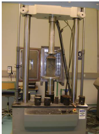
Figure 3.15: Test setup for the determination of the stress-strain relationship
