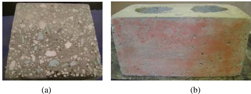
Figure 3.4: the shape and distribution of the HRWR induced air bubbles in the mortar matrix appear on the surface of (a) grinded cube cross section and (b) on the block's surface
