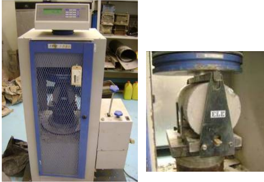
Figure 3.17: Test setup for the Splitting tensile strength tests
