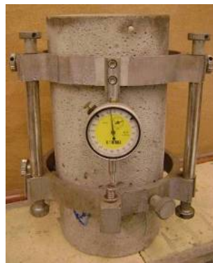
Figure 3.16: The test cylinder fitted with the compressometer
