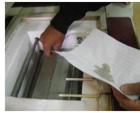
d) : Filling the grooves with the brick powder
