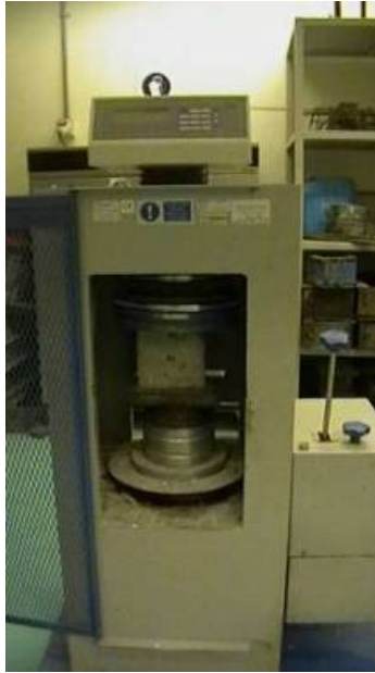
Figure 3.11: Universal testing machine testing cube under compression
