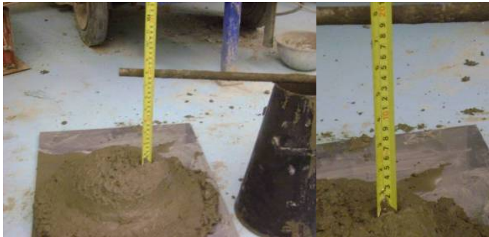
Figure 3.6: HRWR enhanced workability up to a 200 mm slump
