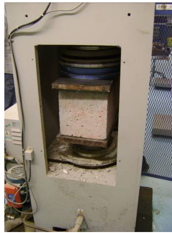
Figure 3.12: Test setup for the EPS mortar hollow blocks
