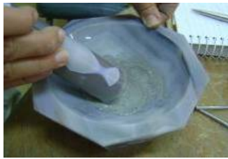
c) : Grinding the debris resulting from engraving the bricks into powder
