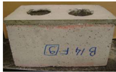
Figure 3.14: EPS Block after capping
