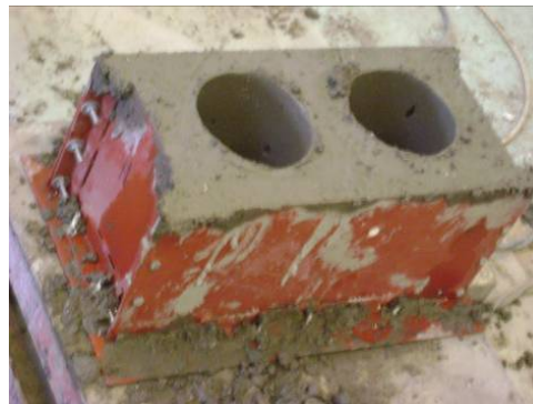
Figure 3.9: The blocks after removing the PVC pipes and leveling the surface
