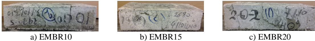
Figure 4.23: Failure pattern of the solid EPS bricks
